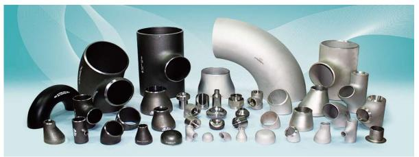
BW Fittings – Elbows & Bends, Reducer (Conc. & Ecc.), Tees (Equal, Reducing & Y-type), Dimensions as per ANSI B16.9, Wall thk. - SCH 10S to SCH XXS Forged Fittings as per ANSI B16.11, SW & Threaded ends, Pressure Class – 3000Cl, 6000Cl, 9000Cl
